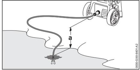
So that the water can be drawn in, the height difference between the pressure washer and the water source should not exceed the maximum suction lift (a),
