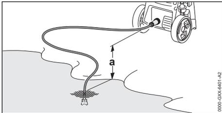
So that the water can be drawn in, the height difference between the pressure washer and the water source should not exceed the maximum suction lift (a),
