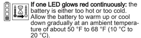
**If one LED glows red continuously:** the battery is either too hot or too cold. Allow the battery to warm up or cool down gradually at an ambient temperature of about 50 °F to 68 °F (10 °C to 20 °C).
