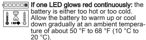
**If one LED glows red continuously:** the battery is either too hot or too cold. Allow the battery to warm up or cool down gradually at an ambient temperature of about 50 °F to 68 °F (10 °C to 20 °C).
