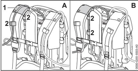
The connecting cord can run through the guide (1) on the shoulder strap (Illustration A), or along the back plate (Illustration B). Secure the connecting cord to the harness with the hook and eye fasteners (2). Always secure the connecting cord using the guide or hook and eye fasteners on the side of the body on which the power tool is held and controlled. Do not allow the connecting cord to swing across your body or hang at your side.
