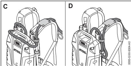
The length of the connecting cord can be adjusted by making a loop around the top (Illustration C) or on the side (Illustration D) of the backpack battery with the hook and eye fasteners.
