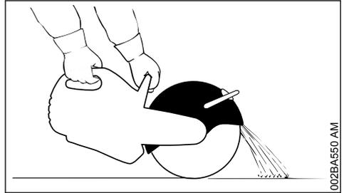
Set the abrasive cutting wheel guard correctly: Guide particles of material away from the user and machine.
