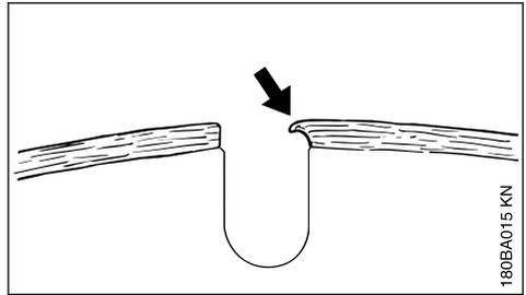
If work continues with dull segments, these may soften due to the high heat generated – the parent wheel is annealed and its strength is compromised – this can lead to stresses that are clearly recognizable by gyrations of the abrasive wheel. Do not continue to use the abrasive wheel – **Risk of accident!**
