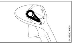
Move the setting lever to 0 – the engine stops – the setting lever springs back to the on position.
