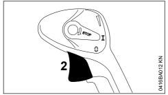
Operate the throttle trigger (2).
