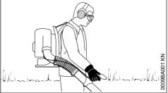
The machine is carried as a backpack. Hold and control the blower tube with your right hand on the control handle.
