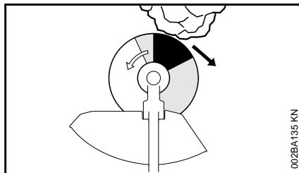
The **risk of kickout is greatest** when the **black area** of the rotating cutting attachment comes into contact with a solid object.
