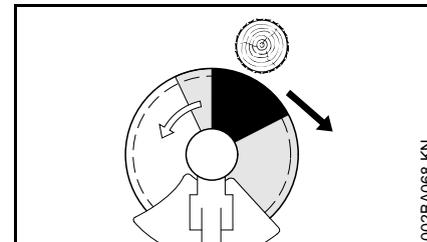
The risk of kickout is highest in the black area of the blade: Do not use this area of the circular saw blade for cutting.
