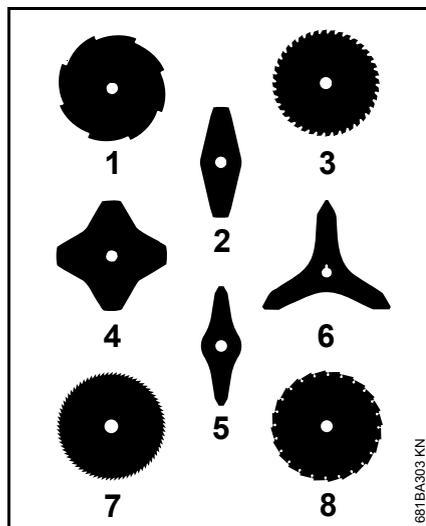
Cutting attachments 2, 4, 5 and 6 may be mounted either way round – they must be turned over regularly to help avoid one-sided wear.
