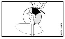
The risk of kickout is greatest when the black area of the rotating cutting attachment comes into contact with a solid object.
