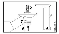
The output shaft (2) must be blocked with the stop pin (6) or screwdriver (6) to mount or remove cutting attachments. These parts come standard with the machine or are available as special accessories.
