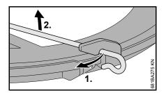
Disconnect wire rod from the transport guard.
