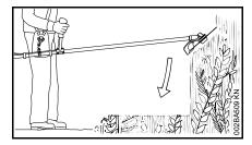
To cut wild growth and scrub, lower the brush knife down onto the growth to achieve a shredding effect – always keep the cutting attachment below hip level during this process.
