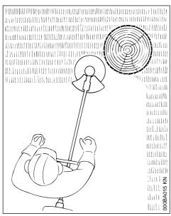
Nylon line achieves a soft cut for edging and trimming around trees, fence posts, etc. – less risk of damaging tree bark.
