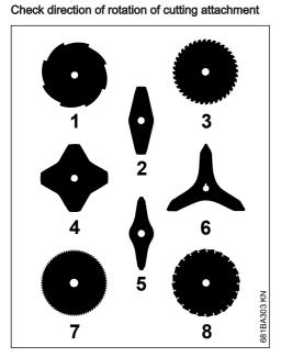
Cutting attachments 2, 4, 5 and 6 may be mounted either way round – they must be turned over regularly to help avoid one-sided wear.
