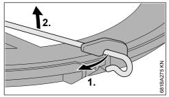
Disconnect wire rod from the transport guard.
