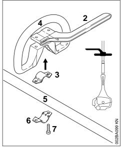
Place the clamp (3) in the loop handle (4) and position them both against the drive tube (5).
