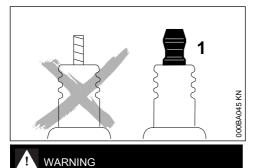
Arcing may occur if the adapter nut (1) is loose or missing. Working in an easily combustible or explosive atmosphere may cause a fire or an explosion. This can result result in serious injuries or damage to property.
