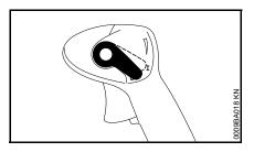
Move the setting lever in the direction of 0 – the engine stops – the setting lever springs back to the on position.
