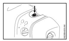
Press the manual fuel pump bulb at least five times – even if the bulb is filled with fuel.
