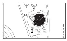
Choke knob automatically returns to the run position I when the throttle trigger is operated.
