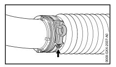
Tighten down the screw (arrow).
