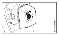
Turn the filter cover lock (1) counterclockwise to the vertical position.
