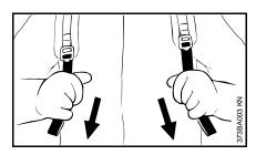
Pull the ends of the straps downwards to tighten the harness.
