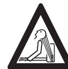
Avoid clothing that could get caught on branches or brush or moving parts of the machine. Do not wear a scarf, necktie or jewelry. Tie up and confine long hair (e.g. with a hair net, cap, hard hat, etc.).
