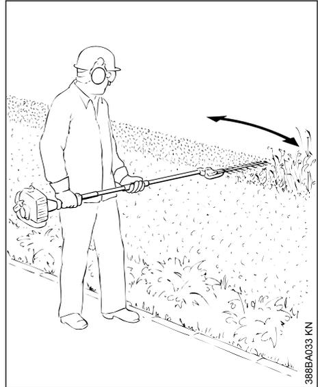
Swing the cutter bar in an arc towards the outside of the hedge so that the cuttings are swept to the ground.
