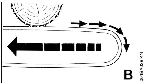
Pushback occurs when the chain on the top of the bar is suddenly pinched, caught or encounters a foreign object in the wood. The reaction of the chain drives the saw straight back toward the operator – **to avoid this risk:**
