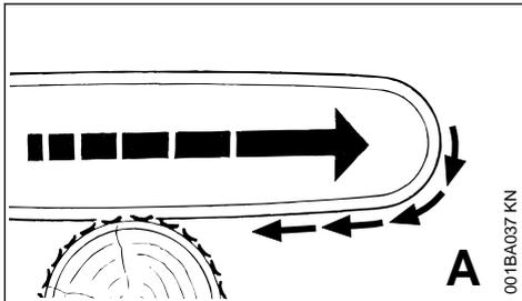
Pull-in occurs when the chain on the bottom of the bar is suddenly pinched, caught or encounters a foreign object in the wood. The reaction of the chain pulls the saw forward – **to reduce this risk, always engage the spiked bumper securely in the tree or limb.**
