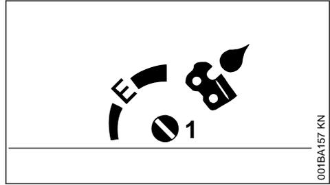
Use the adjusting screw (1) (on underside of machine) to vary the oil feed rate as required.
