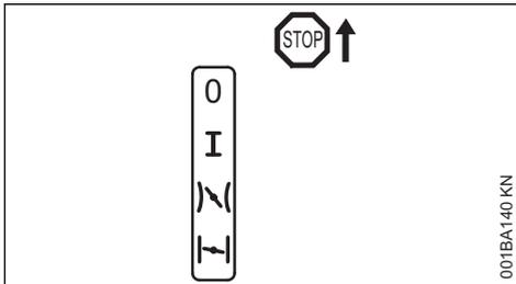
**Stop 0** – engine off – the ignition is switched off
