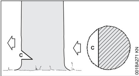
The felling notch (C) determines the direction of fall.
