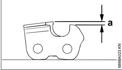
The depth gauge determines the depth to which the cutter penetrates the wood and thus the chip thickness.
