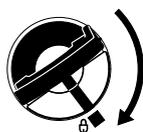
Place the cliplock filler cap (bayonet-type) in position, turn as far as stop and fold the cliplock down.
