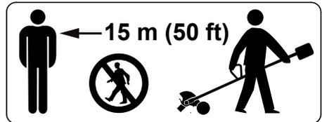
There is a risk of accident from ejected objects within a wide area around the working space, so make sure that there is no-one within a 15 m radius of the power tool. This distance must also be maintained in relation to objects (vehicles, window panes) – **risk of property damage!** Even at distances beyond 15 m, the danger cannot be ruled out.
