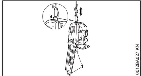
Always use the pull-out ring (4) on the back of the chain saw to transport and secure the chain saw on a rope.
