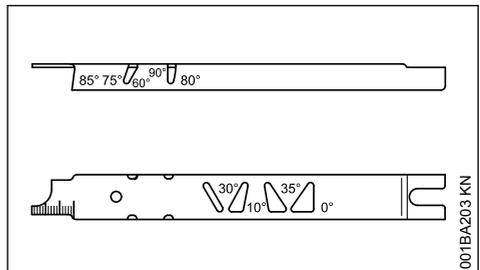
STIHL filing gauge (special accessory, see table "Sharpening tools") – a universal tool for check-
