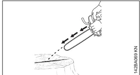
The saw chain must always spin off a small amount of oil.
