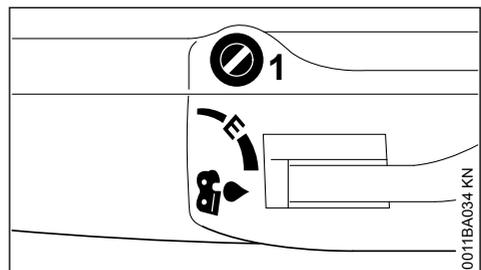
The oil flow can be adjusted as needed using the adjusting screw (1) on the top of the machine.
