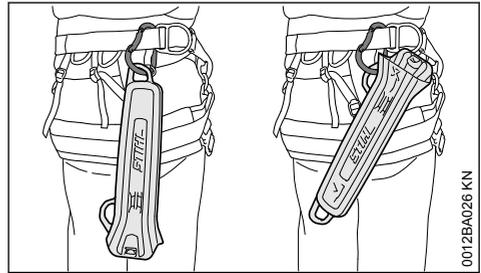
Always use one of the two rings to fasten the chain scabbard to the harness for storage while working.
