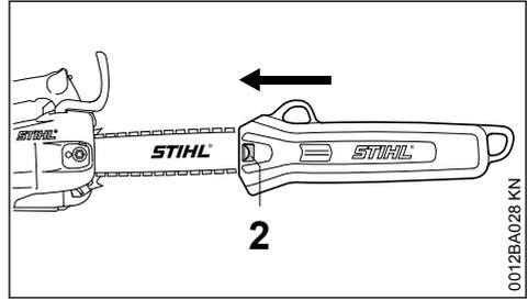
Always push the chain scabbard onto the guide bar as far as it will go. Snap fitting (2) must snap onto the chain sprocket cover.
