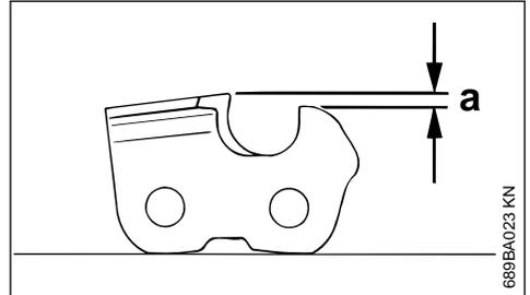
The depth gauge determines the depth to which the cutter penetrates the wood and thus the chip thickness.
