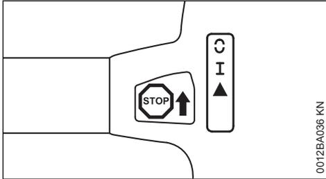
**STOP** or **⊖** – Master Control lever must be pushed in direction of **STOP** or **⊖** to switch off ignition. The Master Control lever springs back to the run position **I** when it is released.
