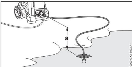
So that the water can be drawn in, the height difference between the pressure washer and the water source should not exceed the maximum suction lift (a),
