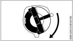
► Hold the fuel cap down and twist it clockwise until it engages
