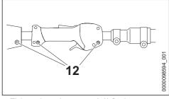
► Tighten down the screws (12) firmly
