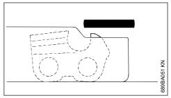
File down the depth gauge until it is level with the filing gauge.
