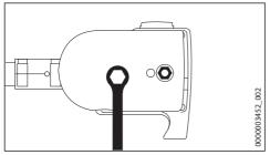
Unscrew the nut and remove the cover
