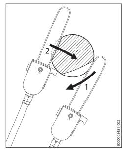
To avoid tearing the bark on thick branches, always start by performing a
