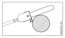
When performing the separating cut, position the bar against the branch near the hook. This will
