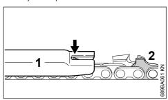
Place a filing gauge (1) that matches the chain pitch on the chain and press it against the cutter – if the depth gauge projects from the filing gauge, the depth gauge has to be lowered.
