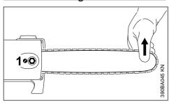
Re-tensioning during cutting work:
