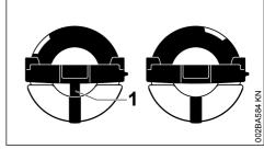
Left: Base of fuel cap is tilted – interior marking (1) is aligned with the exterior marking
