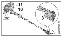
Align the housing (11) (with the manual fuel pump facing up), the control handle (with the stop switch facing up) and the transmission (3) (with the oil tank cap facing up) as shown
