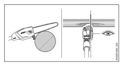
To avoid pinching the saw in the cut, position the bar in the area of the housing against the branch and then perform the cross-cut from the top downward. The saw chain can be positioned precisely using the gauge bar.
