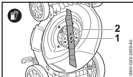
Always check the mounting screw (1) and washer (2) when replacing the cutting blade.
