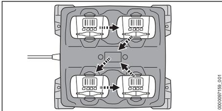
This charger will charge up to four batteries in succession. Charging starts with the battery that is inserted first and follows the pattern shown above. If any particular battery cannot be charged for some reason, that battery is skipped and the charging process continues with the next battery.
