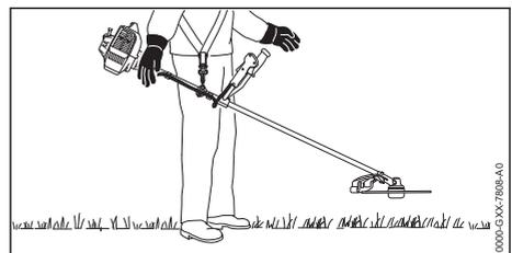
The circular saw blade must hover at a height of about 8 in. (20 cm) above the ground.
