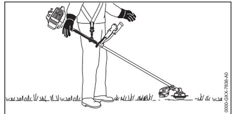
The mowing head or the metal cutting attachment should come to rest gently on the ground.
